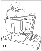
5. Insert the bread pan into the baking chamber. Press down on rim of bread pan until it snaps securely into place **(D)**.
