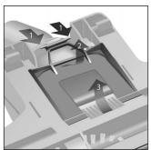
The lower cover can be removed forcleaning the fan and the fan chamber.
