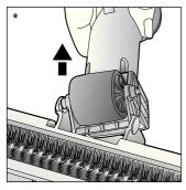
■ When refitting the connector, make sure that it is correctly seated and that it engages correctly in the guide.
