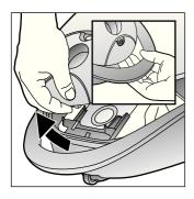
For using the attached micro - filters please insert them into the filter holder which is enclosed.
