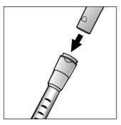
Push the handle into the telescopic tube until it engages.
