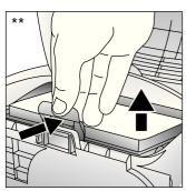
Insert the new micro active carbon filter into the vacuum cleaner and clip into place.
