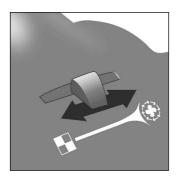
The turbo brush has the possibility to change the rotation speed of the brush from a maximum »A« to a complete stop »B«
