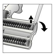
If they are very dirty, e.g. with hair wrapped around them, remove both brush rollers from the hard-floor tool. To do so, lever the rollers out from the side of the guide using a screwdriver, or similar object.
