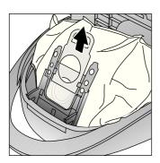
Seal and remove the MEGAfilt\*SuperTEX dust bag by pulling on the tab as shown.
