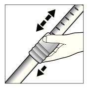
Release the telescopic tube by moving the adjusting sleeve/sliding switch in the direction of the arrow and adjust the tube to the required length.
