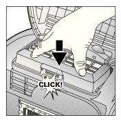
■ Insert the filter holder into the vacuum cleaner and clip into place.
