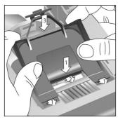
Insert the front lips to reassembly the lower cover
