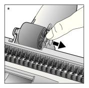
■ The tool connector can be removed if the vacuum channel becomes blocked.
