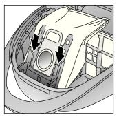
Place a new MEGAfilt SuperTEX dust bag in the holder and close the dust bag compartment lid.
