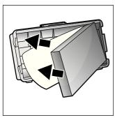
■ Place one of the micro-hygiene filters and the foam in the filter holder.
