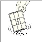
■ Empty the motor protection filter by tapping it.
