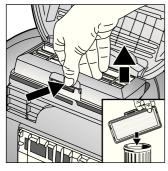
Unlock the exhaust filter by pushing the locking tab in the direction of the arrow and remove it from the vacuum cleaner.
