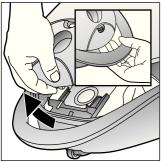
Open the cover by moving the locking lever in the direction of the arrow.
